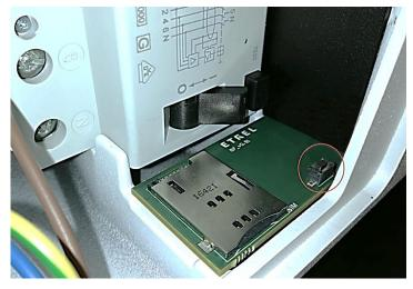
Figure 8: Reset button inside the maintenance opening
